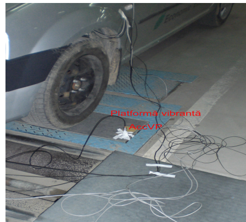
Fig. 4 Detail regarding the suspension, the positioning of the transducers and of front wheel on the oscillating platform
